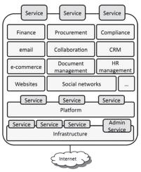
Figure 2 Software-as-a-Service (SaaS) Stack
