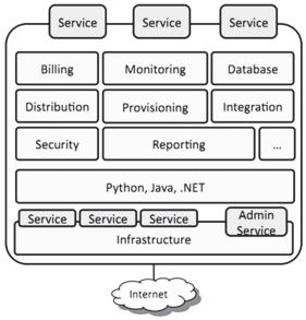
Figure 3 Platform-as-a-Service (PaaS) Stack
