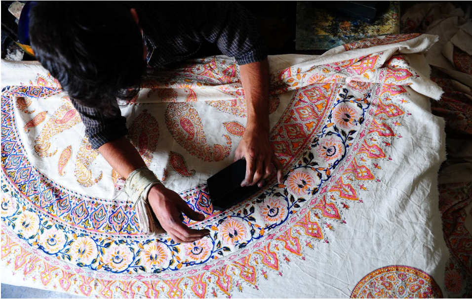
In the above picture, an artisan is carrying out traditional calico block printing. The term 'calico' is used to refer to a plain-woven textile which is made from unbleached and often not fully processed cotton. Calico printing is the process of printing and making fast – colour designs on calico fabric. — The Encyclopedia of Crafts in Asia Pacific Region
