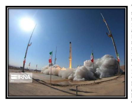
The Zuljanah is a threestage rocket, with a solid-fuel engine in the first and second stages and a liquid-fuel engine in the third stage. It needs to complete a few more tests to become fully operational. When that happens, the SLV would be capable of launching satellites weighing up to 220 kilogrammes to altitude of 500 kilometres above the earth's surface.
